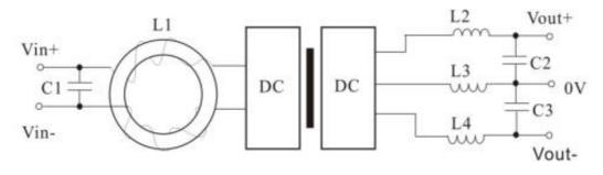
$\equiv$ .DC-DC module converter isolation withstand voltage test method
