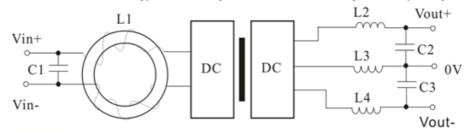
DC-DC Converter isolation withstand voltage detection method.
