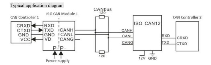
The above picture is a typical application diagram of ISO CAN. Conventional circuits require CAN isolation transceivers that are realized by a combination of optocouplers, DC/DC isolated power supplies, CAN transceivers and other components. Now a low cost, small volume SIP8 packaged ISO CAN module can be completely replaced, and SIP12 packaged Isolated power distribution output 3.3V/5VDC, which can supply power to the board, making it easier to use.
