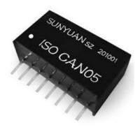
Single in-line 8-pin package: SIP8 Pin
