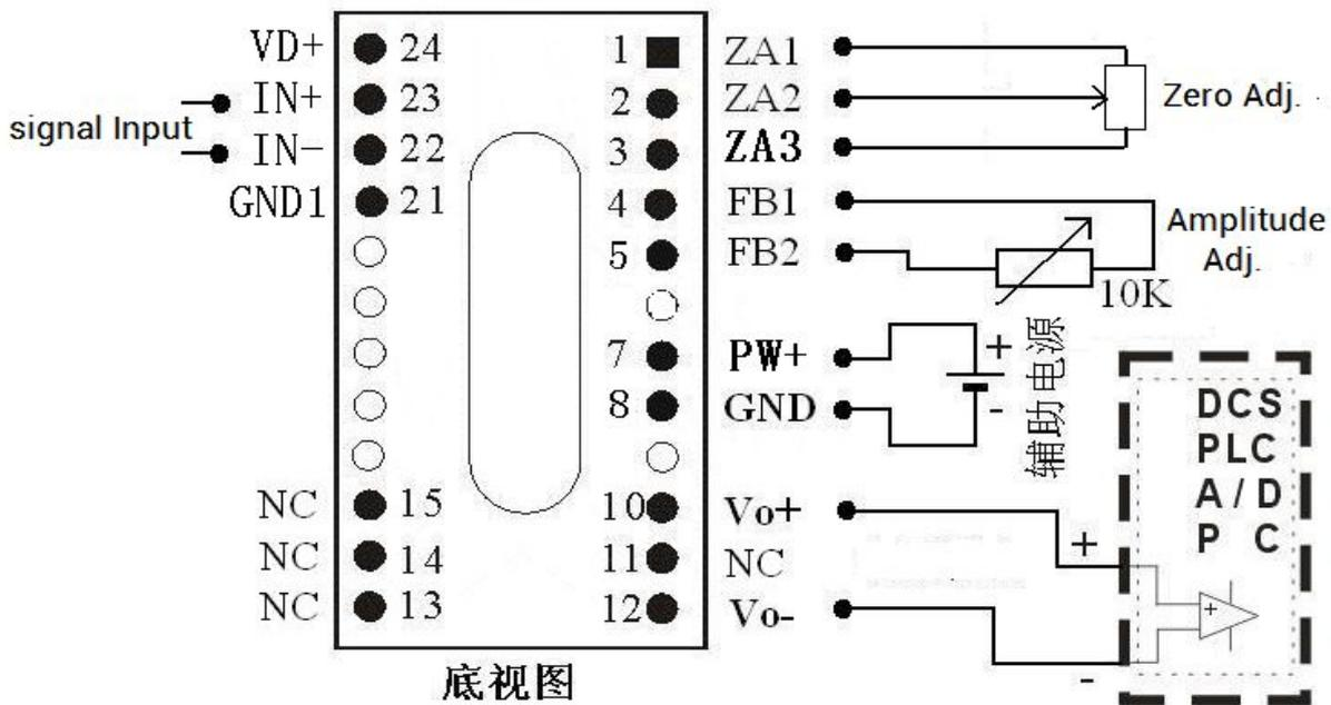
Voltage Signal Output Transmitter PIN Description: DIP 24 Pin Package with Gain/Zero Adjustment
