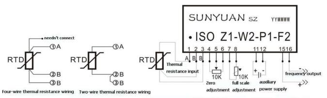
Typical application diagram of voltage pulse output (fixed voltage pulse output)
