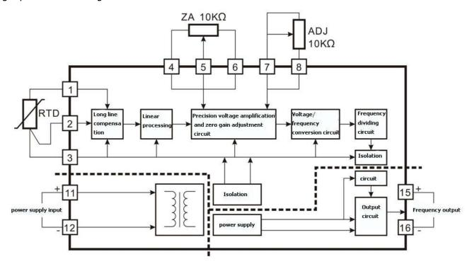
Picture 1 ISO Z-W-P-F Series Isolation Transmitter Block Diagram
